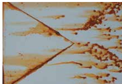
Corrosion resistance on cold-rolled steel after 520 hours of Salt Spray Test Paint based on control latex
