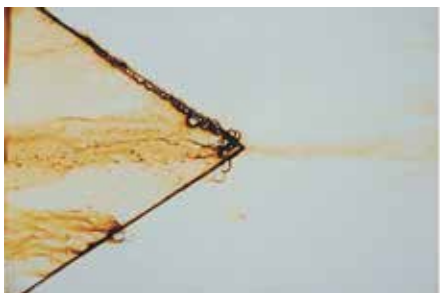
Corrosion resistance on cold-rolled steel after 520 hours of Salt Spray Test Paint based on S/A latex with 1% Sipomer PAM-200
